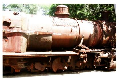
The locomotive was a ZE class, commissioned in the year 1950 with 2-8-2, wheel arrangement. The engine weighed 35 tons and the tender weighed 10 tons. This loco was condemned in the year 1995. Since then it was left exposed to the vagaries of nature.
